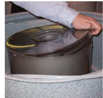
How to remove the clear lid from the Eazy. This is a tight fit. Do not remove the screws
